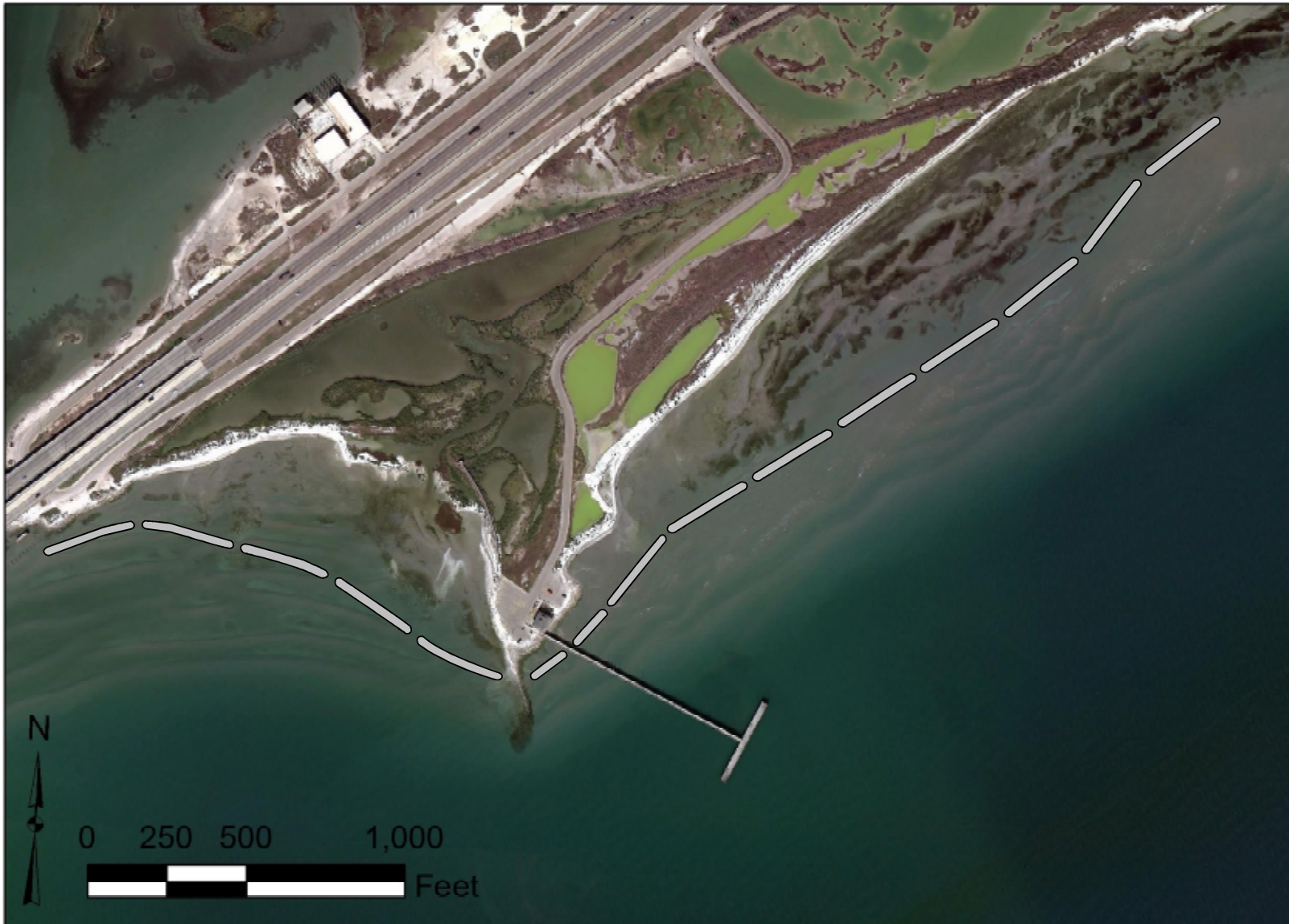
Figure 3.3 Alternative 3: Segmented Breakwater with Continued Breakwater Alternative at Point (Conceptual).
