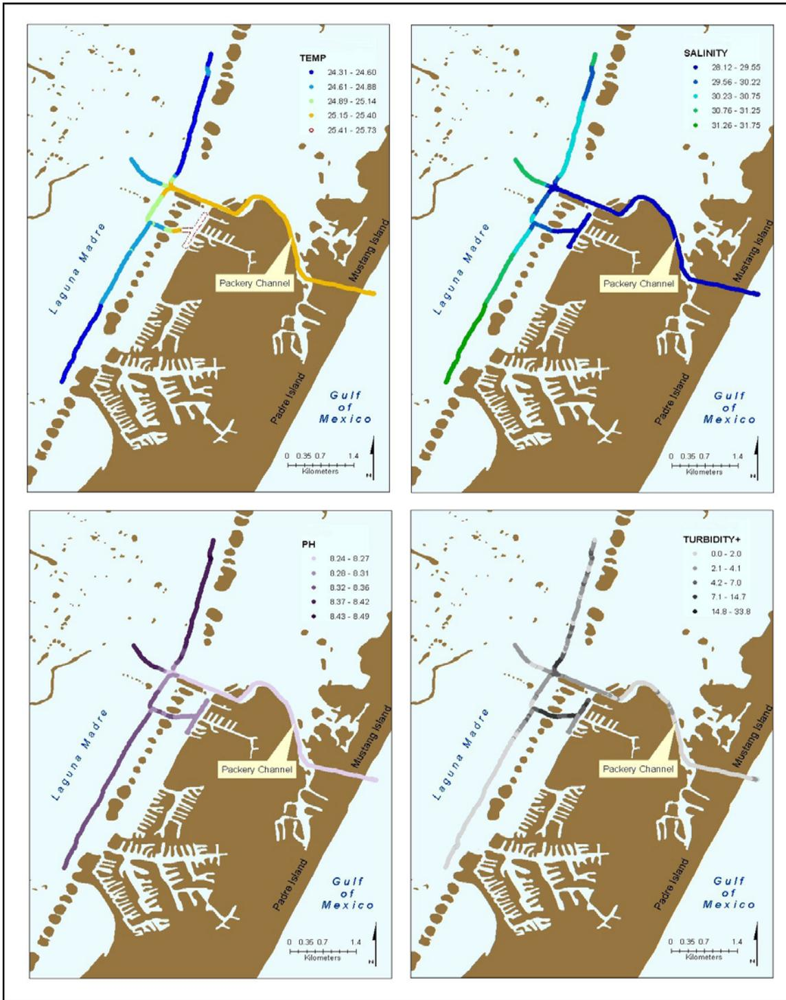
Figure 3. Graphical representation of water quality survey results from the Packery Channel region of the Upper Laguna Madre. Panels show color coded representation of the spatial distribution of temperature, salinity, pH, and turbidity on 20 May 2007 (Survey 2).
