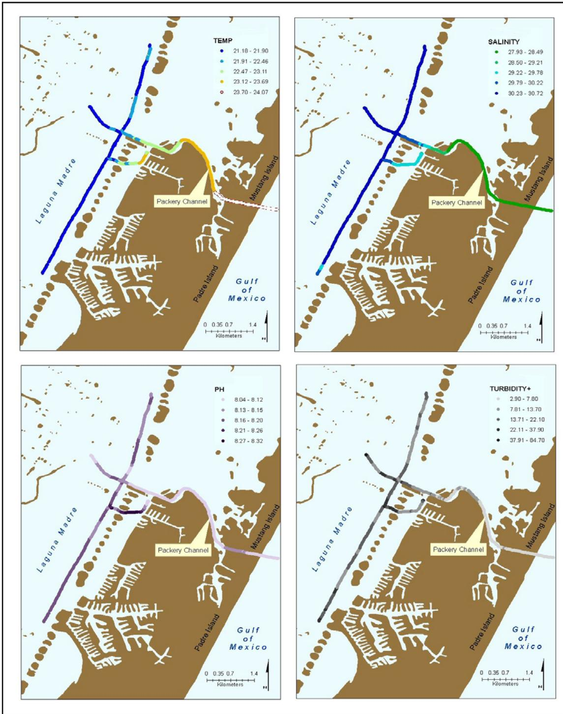
Figure 5. Graphical representation of water quality survey results from the Packery Channel region of the Upper Laguna Madre. Panels show color coded representation of the spatial distribution of temperature, salinity, pH, and turbidity on 29 April 2008 (Survey 6).
