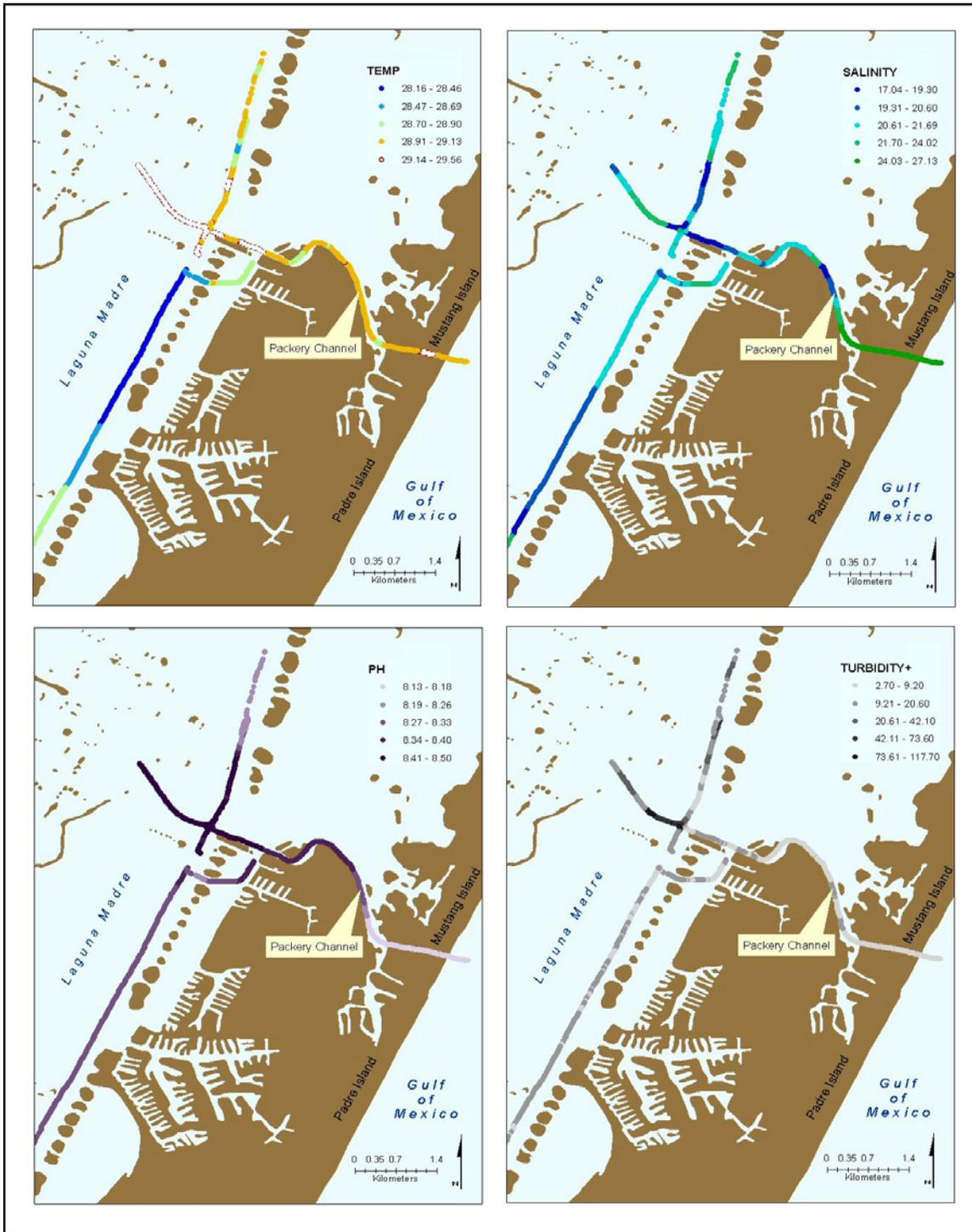
Figure 7. Graphical representation of water quality survey results from the Packery Channel region of the Upper Laguna Madre. Panels show color coded representation of the spatial distribution of temperature, salinity, pH, and turbidity on 08 October 2008 (Survey 4).
