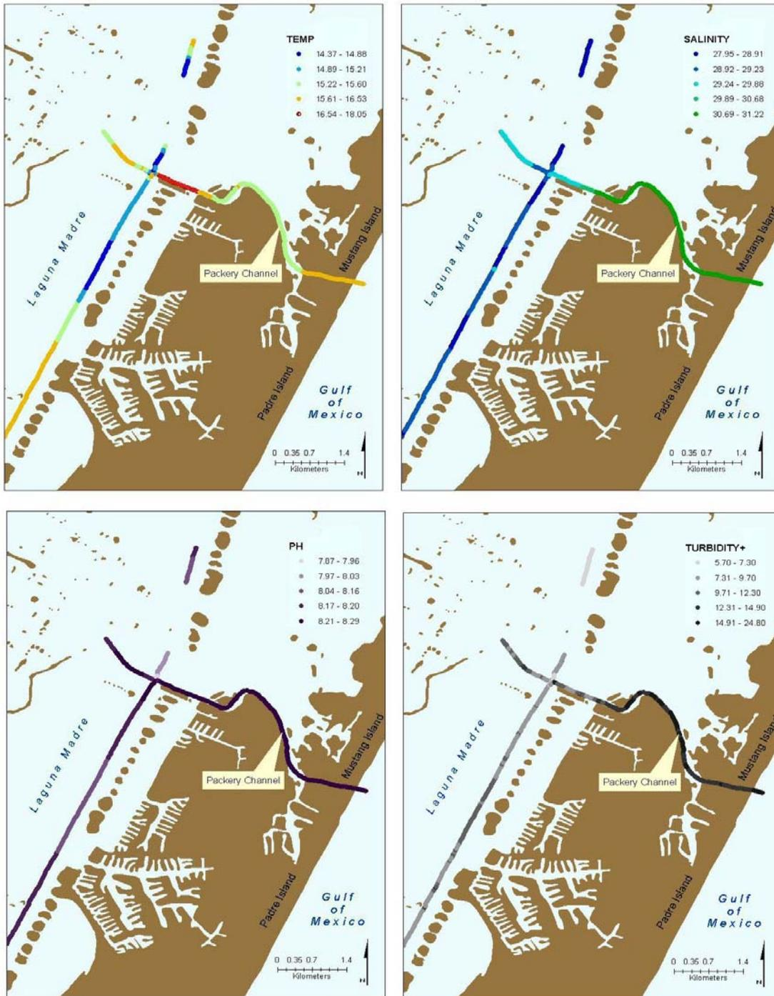
Figure 4. Graphical representation of water quality survey results from the Packery Channel region of the Upper Laguna Madre. Panels show color coded representation of the spatial distribution of temperature, salinity, pH, and turbidity on 13 February 2008 (Survey 5).
