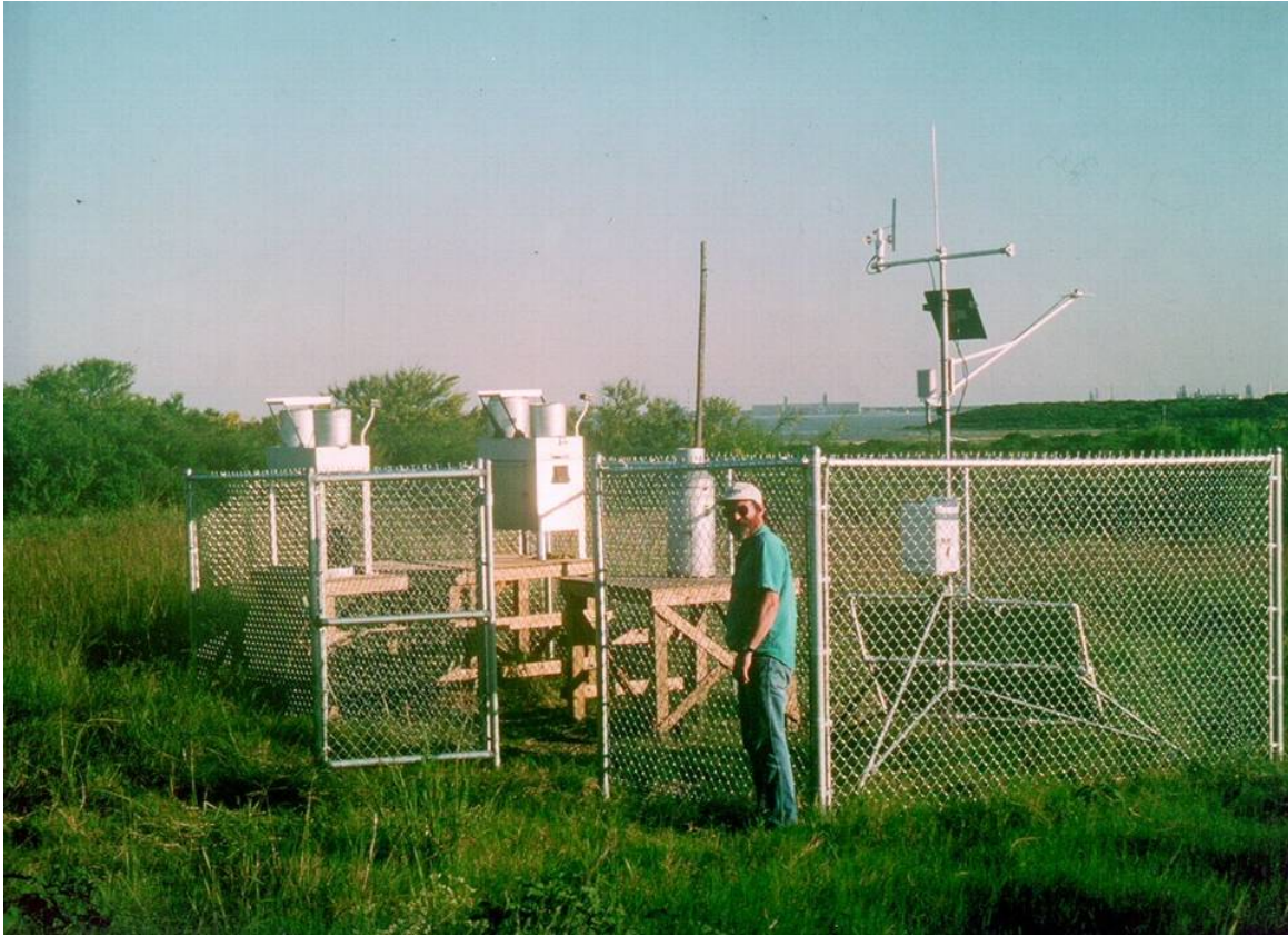
Figure 2. Whites Point Atmospheric Deposition Sampling Station, Note the Two AeroChometric Samplers, the Belfort Rain Gauge, and the Meteorological Sensors Located in a Fenced Enclosure across from the Refineries in the Background.
