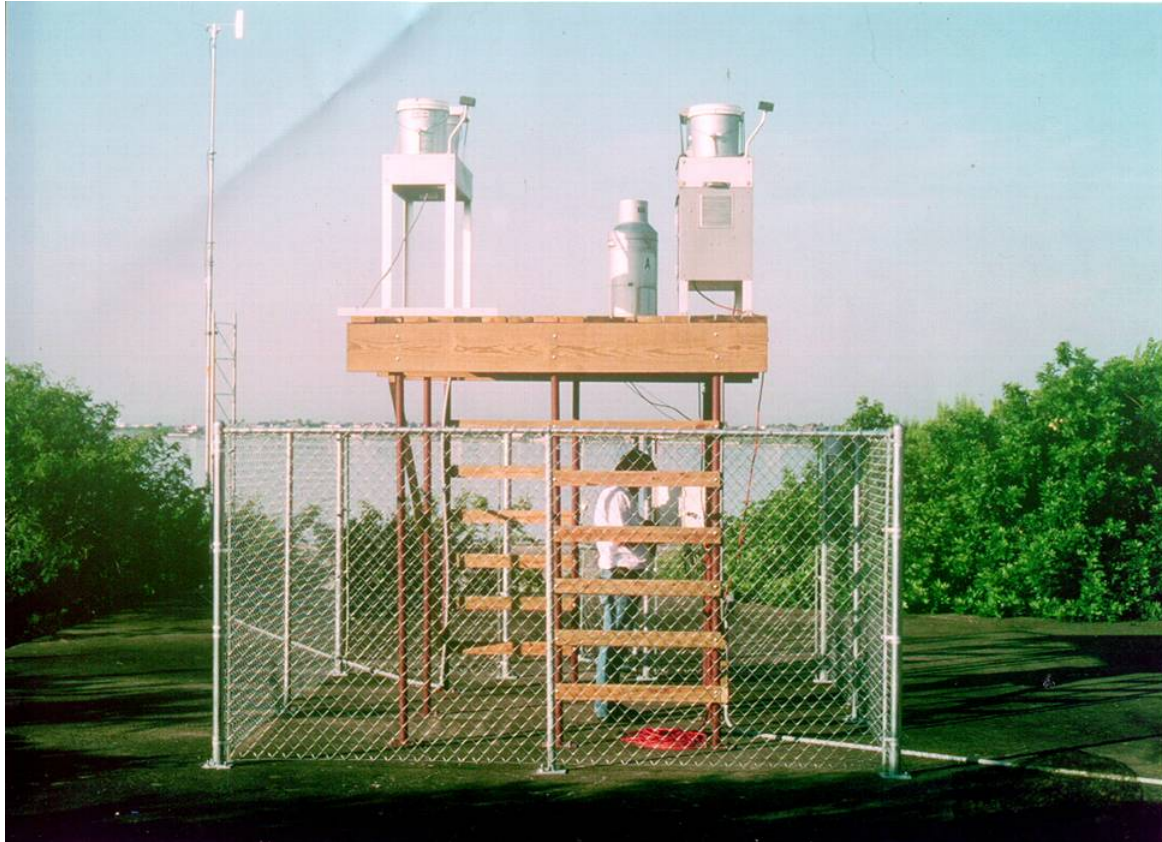
Figure 3. Texas A&M Corpus Christi Atmospheric Deposition Sampling Station, Note the Two AeroChometric Samplers, the Belfort Rain Gauge, and the Meteorological Sensors Located in a Fenced Enclosure with Oso Bay in the Background.
